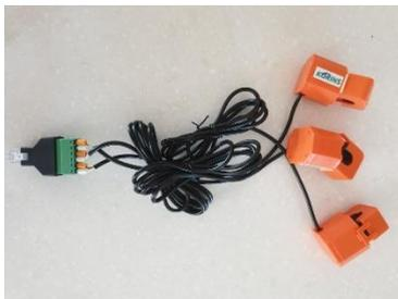
if you see "--" data on lcd display, please rotate the clamp connecting position
