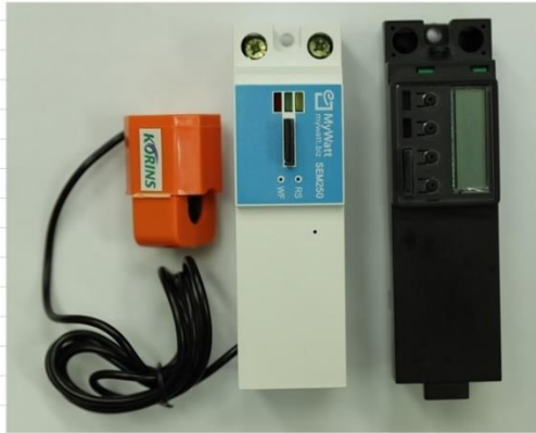
SEM250WIFI Single Phase 3-channel Energy Logger
